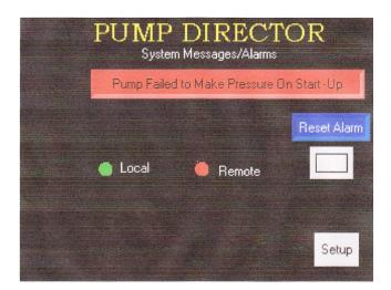
The alarm condition will remain 'locked in' until the **Alarm Reset Pushbutton** is depressed or a remote alarm reset input signal (momentary dry contact closure) is received on terminals I8 and +24 (remote alarm reset only permitted with L-O-R switch on the Pump Director Door is in the Remote position). Note that turning the L-O-R switch to the Off position will not reset an alarm condition.
