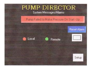
The alarm condition will remain 'locked in' until the **Alarm Reset Pushbutton** is depressed or the alarm is reset by remote alarm reset input signal.
