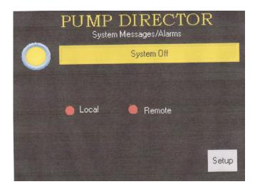
When the Standby Screen is visible, only the **Setup Pushbutton** is available. Pressing the **Setup Pushbutton** will cause the **Setup Screen** to become visible:
