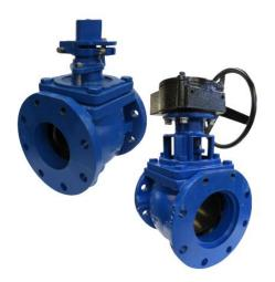
125/150 flanged ends for exposed installations. Plug valves are designed with eccentric rubber disc seating surfaces. The plug rotates 14 turn to provide shutoff in pipes. Tighter shutoff is provided by the eccentric seating action as the actuator is adjusted to provide for more rotation. The valve can be adjusted to a maximum of 10 degrees over travel. Pipeline flow can be regulated by positioning the plug between 15 and 90 degrees open.
