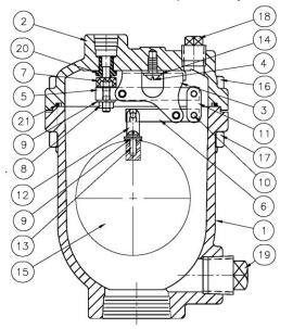
Lubricate and place O-ring (21) in cover (2) and carefully place cover (2) on body (1) ensuring o-ring is retained. Install the cover bolts (16) and nuts (17) and tighten in an alternating pattern.
