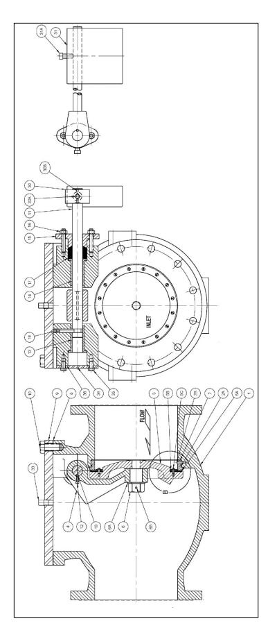
Figures 220-D, 220-DS, 220-U and 220-US Lever & Weight Swing Check Valve Parts Location
