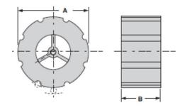
Class 125/150 flange bolts fit in grooves, Class 250/300 flange bolts fit outside grooves
