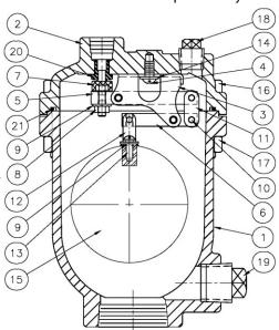
Lubricate and place O-ring (21) in cover (2) and carefully place cover (2) on body (1) ensuring oring is retained. Install the cover bolts (16) and nuts (17) and tighten in an alternating pattern.
