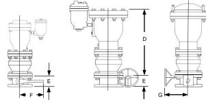
Standard NPT Outlet Optional Flanged Outlet or Standard Outlet Cowl (Inlet Isolating BFV Available only 3" to 10" Class 125 Flanged Inlet Only)
